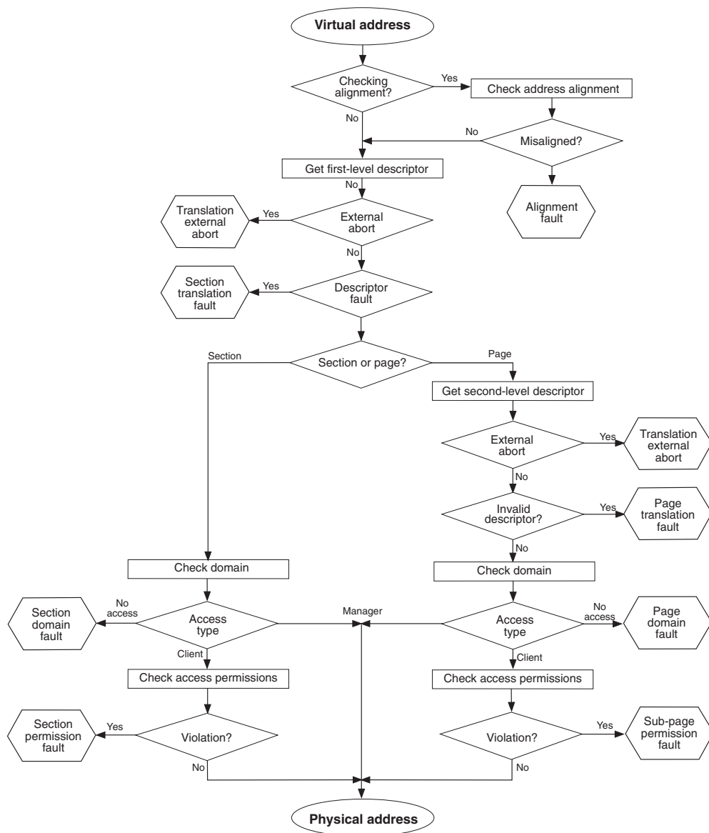
Figure 3-9 Sequence for checking faults
