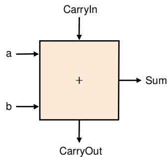
$$\begin{aligned}C_{\text{out}} &= a \cdot b + a \cdot c_{\text{in}} + b \cdot c_{\text{in}} \\ \text{sum} &= a \oplus b \oplus c_{\text{in}}\end{aligned}$$
