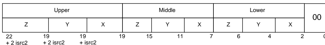
FIGURE A-4 Three-Dimensional Array Blocked-Address Format (Array32)
