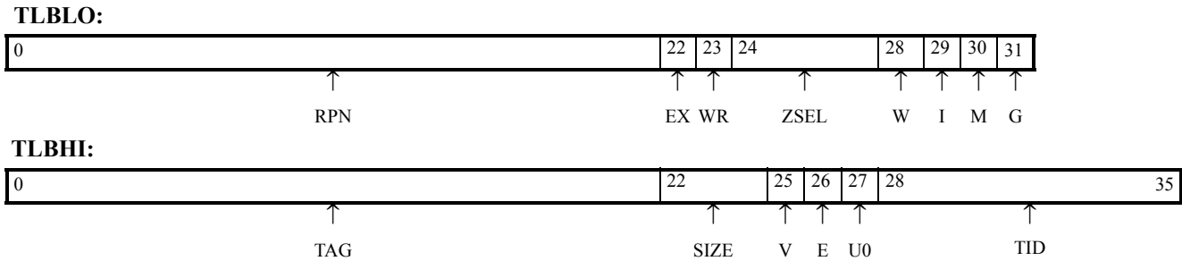
Figure 1-18: TLB Entry Format
